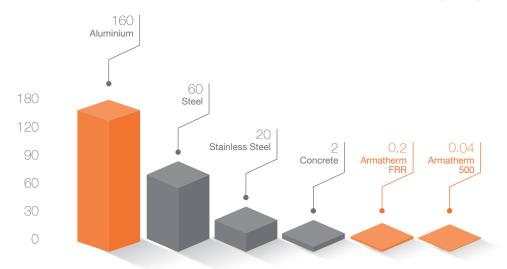
Thermal conductivity values of Armatherm™ structural thermal break materials as compared to standard building materials.
