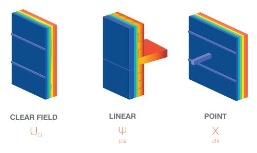
Examples of thermal transmittance and heat flow through the building envelope. Steel girts can be seen in the clear field wall assembly, a steel shelf angle bolted to a slab edge as an example of a linear detail and a single beam penetrating the envelope as a point detail. (Source: Morrison Hershfield)
